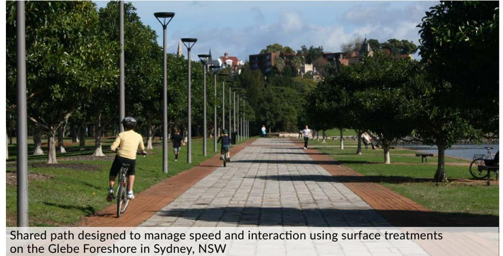
Shared path designed to manage speed and interaction using surface treatments on the Glebe Foreshore in Sydney, NSW
